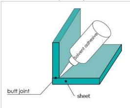
As the solid content of such glues is low, they have no joint filling capability. When bonding the sawn edge, smoothing the surface to be bonded using sharp edge scraper can reduce possible bubble formation.
