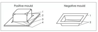
such as wrinkle or web formation (2) and shock marks, can be solved by adequate pneumatic stretching prior to final "pull down. High tool temperatures and high tool speed can also cause shock marks. Negative forming means that the semi-finished sheet is drawn into the mould cavity. This is sometimes called "female" forming. Thin corner areas (2), which may appear during negative forming of sharp-edged components, can be reduced by mechanical top die stretching.
