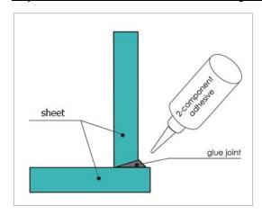
The pasted seam must be prepared by chamfering; this does not apply to butt joint bonding. The adjacent sheet area must be masked with an adhesive compatible tape. The adhesive must be mixed as prescribed by the adhesive supplier. Removal of bubbles in vacuum is possible.
