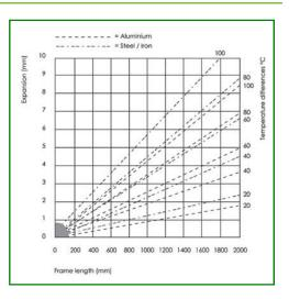
POLYCASA PC shows a coefficient of thermal expansion of 0.065 mm/m o°C.
