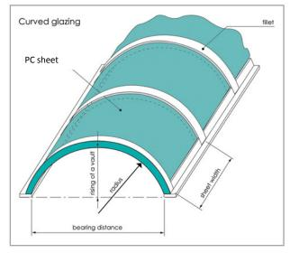
Supporting bow spacing: max. 2000 mm; Average expansion level: 5 mm/m.
