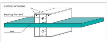
bending zone. If bending is performed too cold, stresses will be created that will result in a brittle part.
