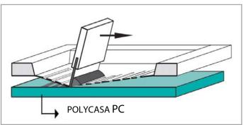
Distortion screen printing allows the flat sheet to be formed after printing into a three dimensional article with correct print register. Allowance must be made for "stretching" of the image when designing the graphics.
